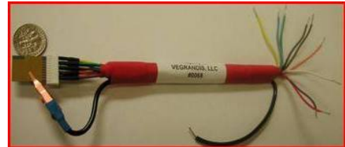
Figure 2. Digital photo (top) of the VEG 4X1™ Connector and the VEG 4X1™ chip.
